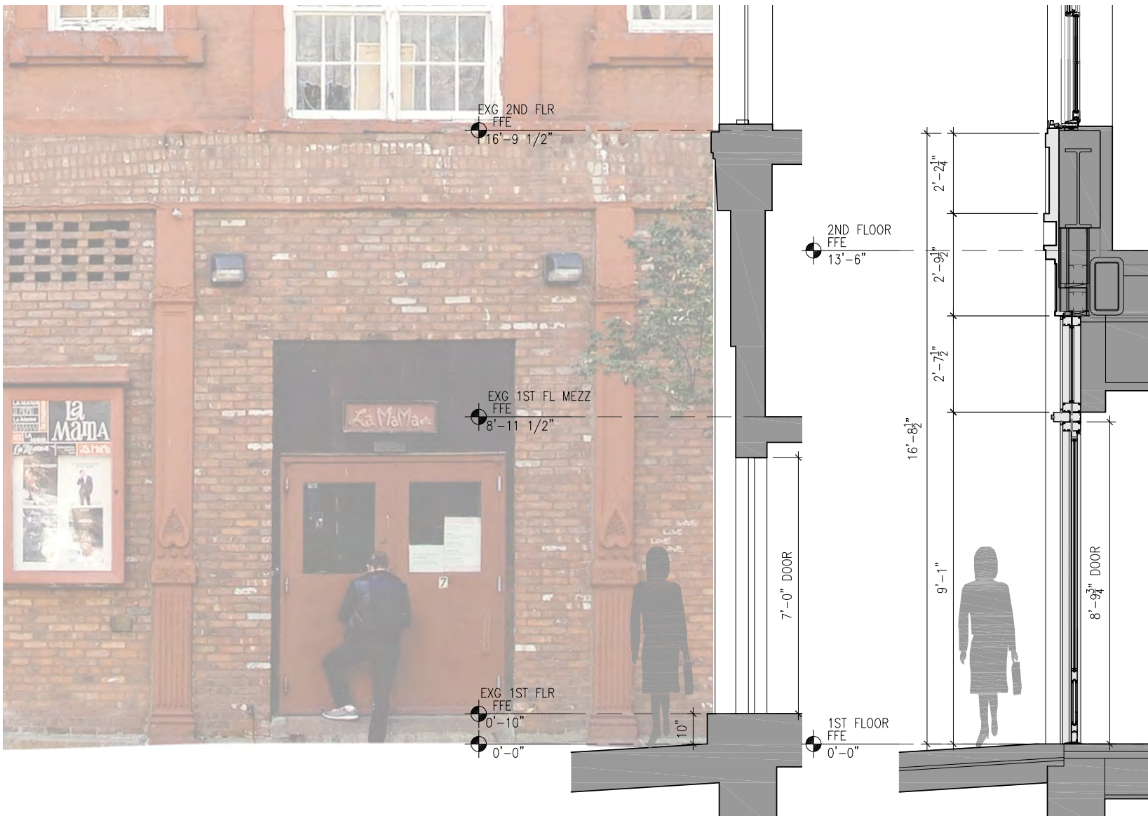
EXISTING SECTION AT 1ST FL W/ SUPERIMPOSED ELEVATION
